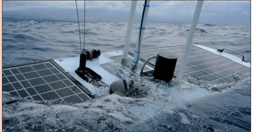
*Wave Glider surf board with solar power and communications, attached to drone below the surface*
